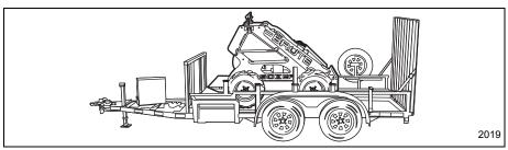
Figure 3-10 Transport Position on Trailer
